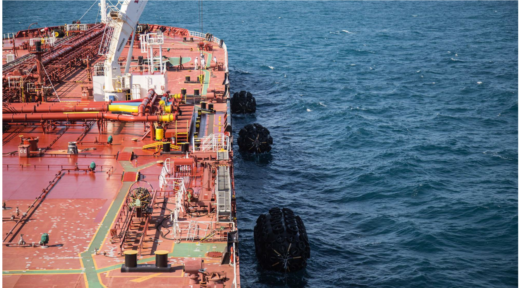
A constant heading tanker with fenders already in place awaiting the maneuvering tanker.
