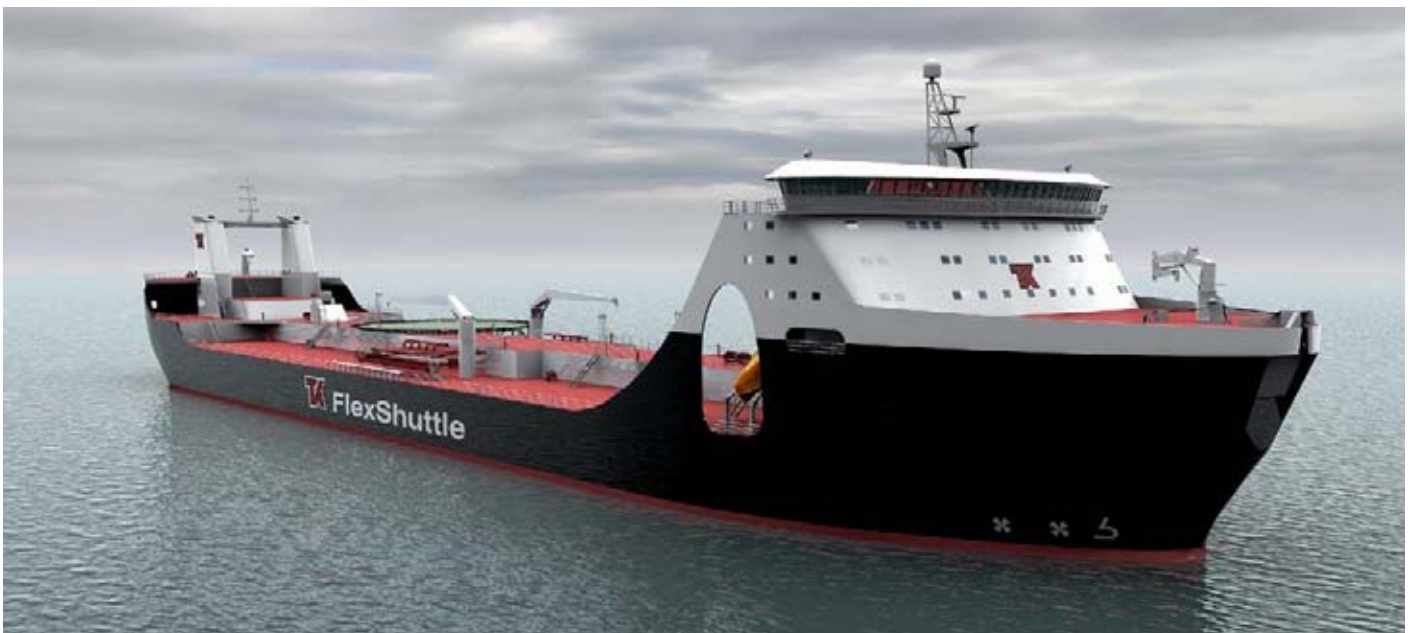
Teekay FlexShuttle stern-loading Shuttle Tanker Design
